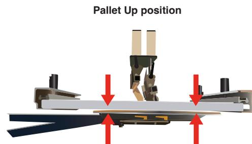
4. With your pre-sheered ink in your screen, a test garment or Pellon® loaded onto the press, squeegee angle set at 15 degrees, pressure set at 35–40 PSI, and a 60/90/60 or 70/90/70 squeegee installed, you are ready for your first test print. Perform your first test print. As long as everything goes as expected, do one or two more strokes to ensure the stencil gasket is loaded with ink, and replace your test material with a new Pellon or test garment.
