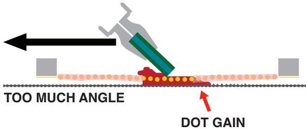
On automatic presses, start with a squeegee angle between 10–15 degrees. On manual presses, begin holding the squeegee behind your ink deposit while resting the blade on the screen surface. From a vertical position resting squarely on the foot of the blade, add downward pressure while beginning to lean the squeegee handle back. Begin your pull, ensuring not to lean the squeegee handle back very far.
