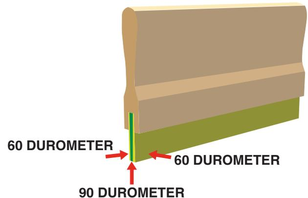
The outside durometer helps to create a softer, smoother ink deposit and is less likely to disturb surface fibers. White inks and inks with high white content, like yellows, benefit from 60/90/60 squeegees. For dark inks, 70/90/70 helps to hold finer detail.
