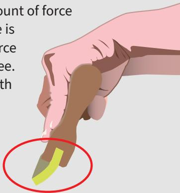
Do not hold the squeegee from the sides, as this technique will add a curve to your blade and create an uneven ink deposit. This technique will also usually result in excess of print pressure and produce fibrillation or distorted prints.
