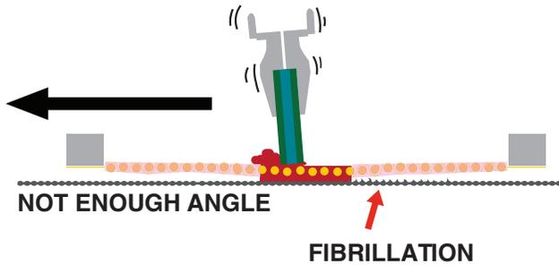
Too little angle can create what is known as “chatter,” leaving undesired lines in the print deposit. It can also cause fabric surface disturbances and fibrillation.
